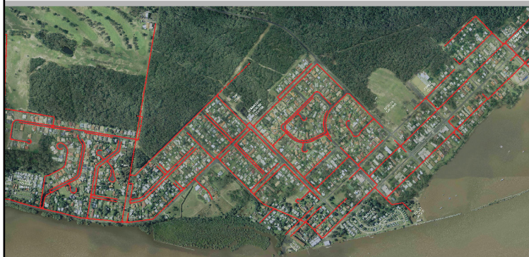
Caption: PS Solutions design layout for Iluka Pressure Sewerage Scheme (2,100 Ultimate Lots)
